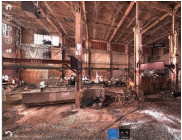
MEASURED APPROACH To assist the construction team (left), a laser scan was performed and utilized to create a three-dimensional digital model from which exact measurements could be obtained at any elevation within the existing structure (right).
